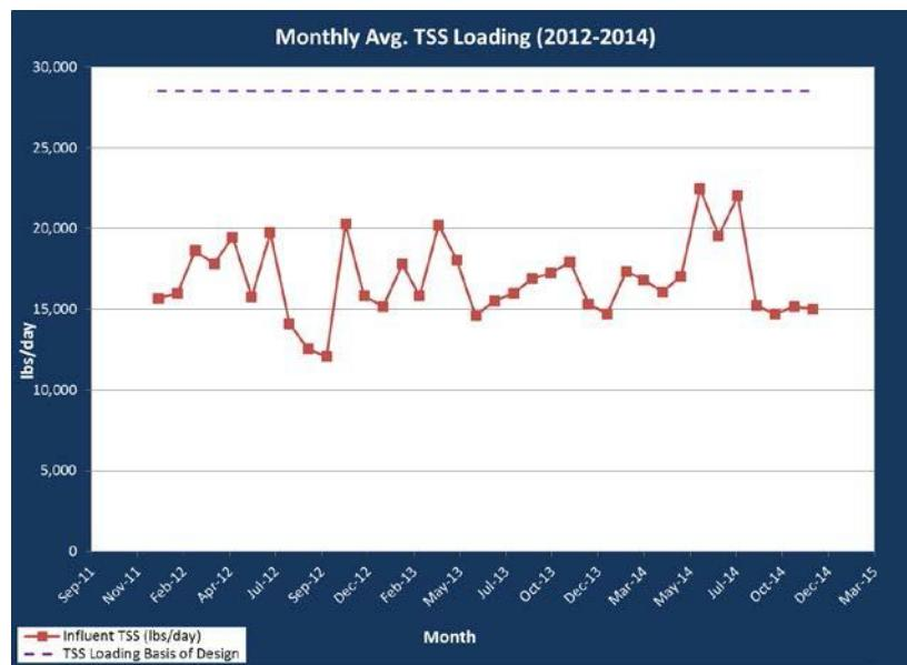
Monthly average mass loadings of total suspended solids in the influent flow was also comfortably below the plant's design loading of 28,520 lbs/day throughout the period.
